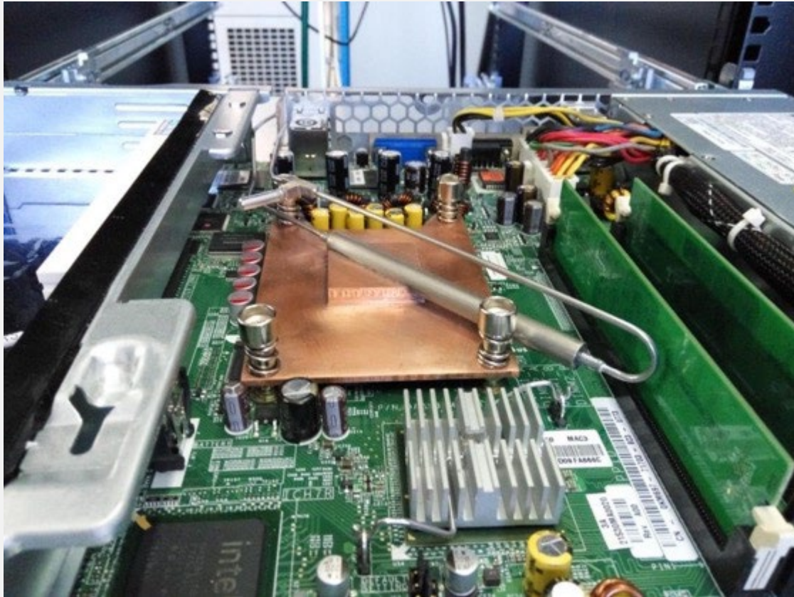
Replacement of the heat sink with the interface
