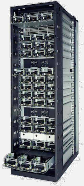
Open Rack V2 (45 servers)
